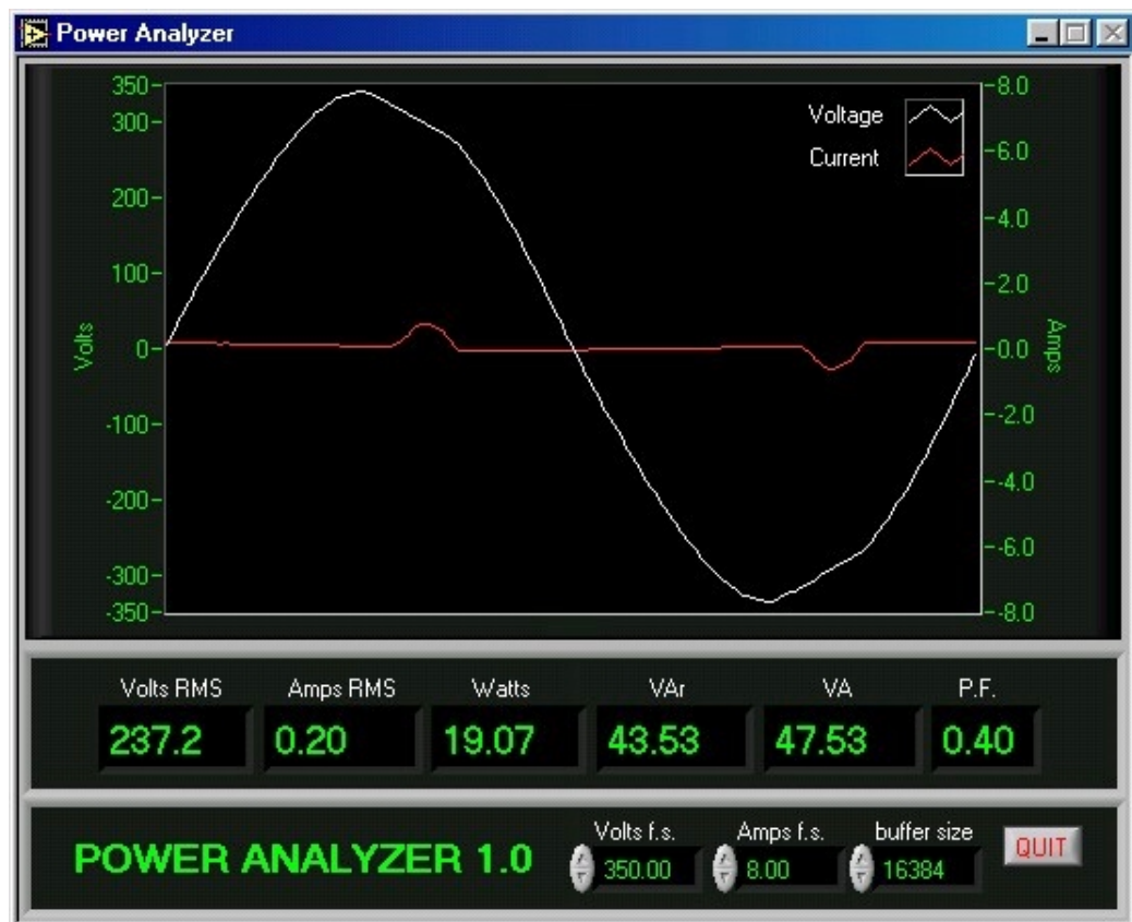
(Fig. D.5: Power analysis of mains power unit of a laptop)
