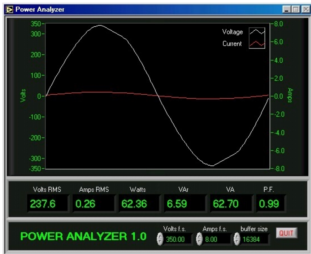
(Fig. D.4: Power analysis of 60-watt light bulb)
